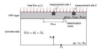
Figure 1 Delamination of a FRP layer bonded to a concrete slab.
